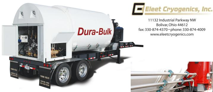
Dura-Bulk uses a hydraulic pumping system that provides extremely high flow, high pressure pumping capabilities with easy access for periodic maintenance. Our unit does not include the PLC with automatic pump shutoff. We have also eliminated many of the fragile electrical components that tend to fail. This ensures trouble free continual operation for years to come. For more information, visit www.eleetcryogenics.com, or call 330-874-4009.
